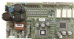
Escalator Extension Board
