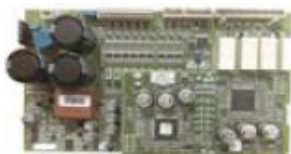
Escalator Extension Board
